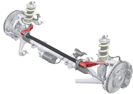
Fig. 1: Chassis stabiliser as a driving dynamics component for influencing the roll and steering behaviour of the vehicle (Source: Audi AG)
