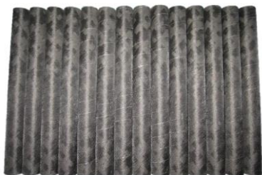
Fig. 3: FilaWin® 50k samples with a \pm 45^\circ lay-up
